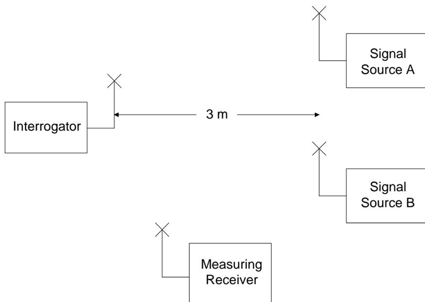
**Figure B.4: Radiated measurement of blocking**
