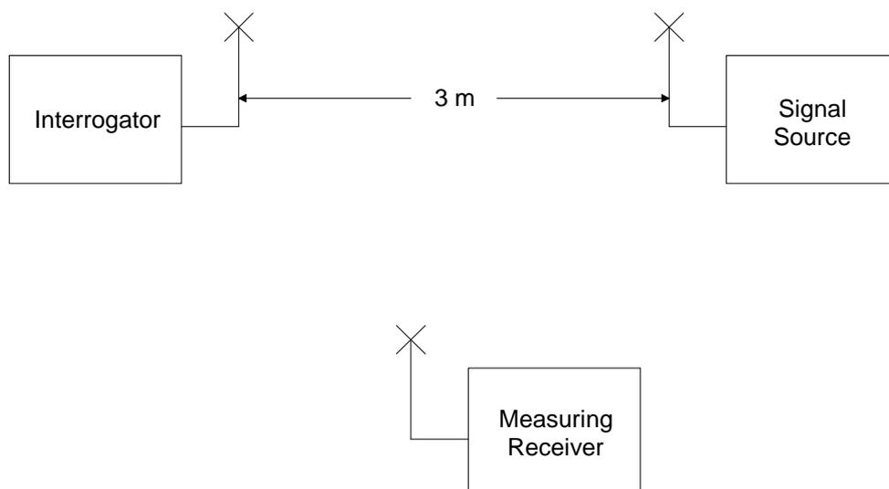
**Figure B.2: Measurement of threshold level**
