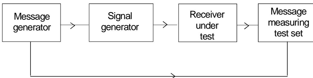
**Figure 3: Measurement arrangement**
