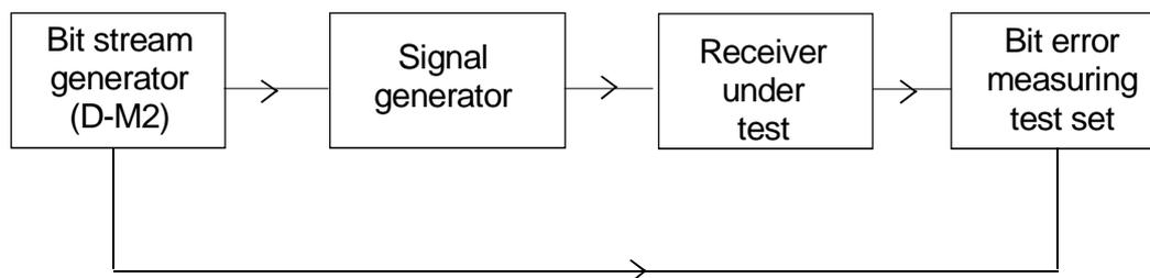
**Figure 2: Measurement arrangement**
