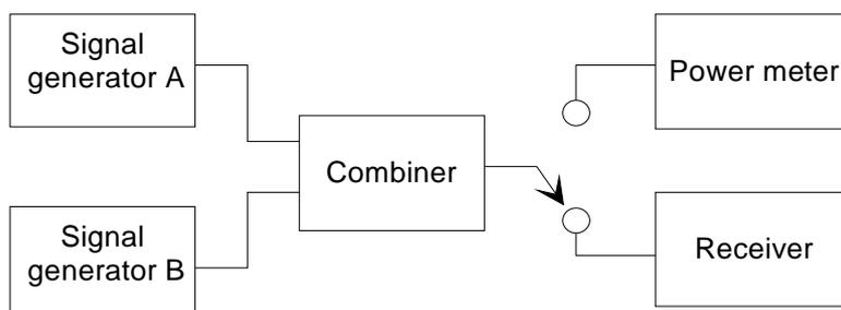
**Figure 8: Measurement arrangement**
