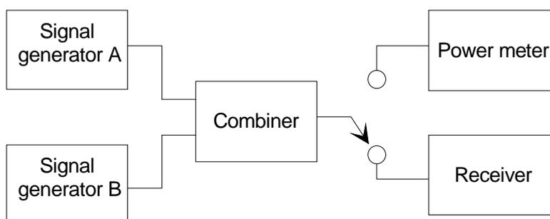
**Figure 5: Measurement arrangement**
